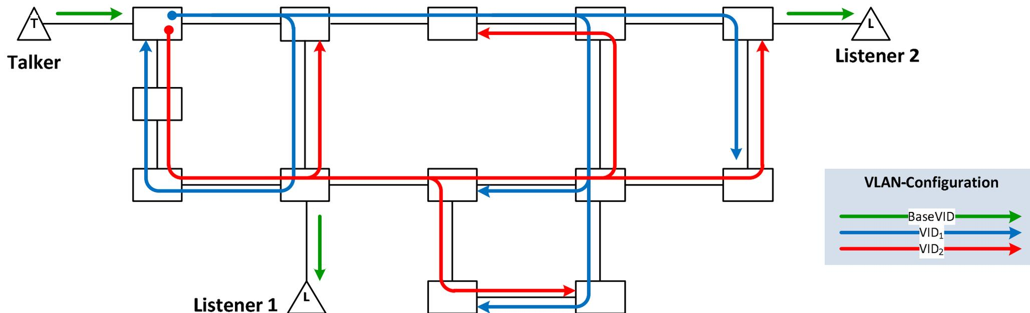
1. One VLAN with a BaseVID (“green”) and **two** associated VIDs for the maximal redundant trees (“red” and “blue”), e.g. installed by ISIS-PCR (è MRT)
