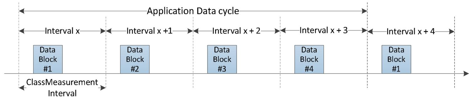
Example: adaption of application data cycles to network class measurement intervals at end-stations using “reduction-ratio”
