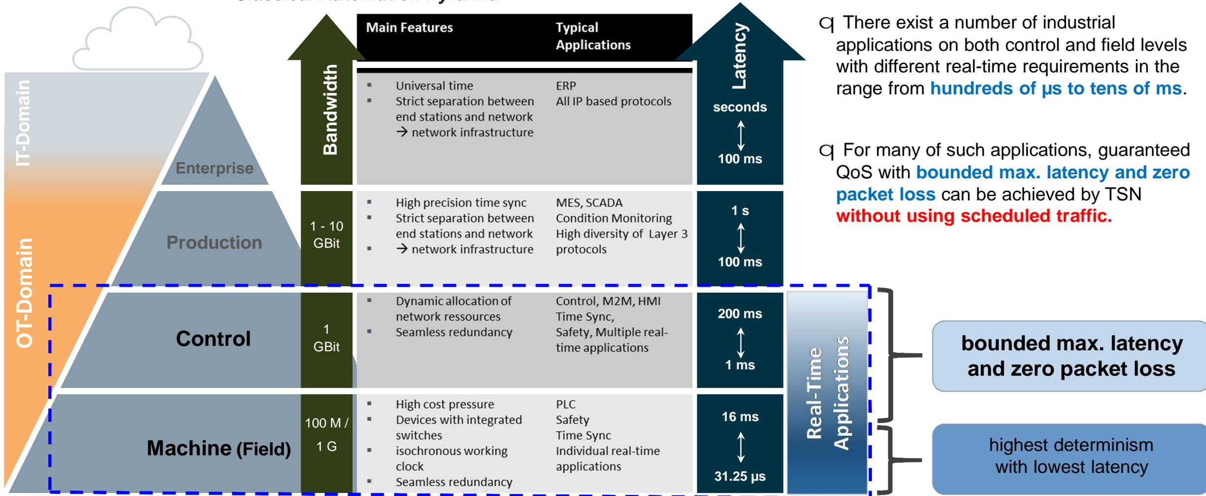
Q There exist a number of industrial applications on both control and field levels with different real-time requirements in the range from **hundreds of μs to tens of ms.**
