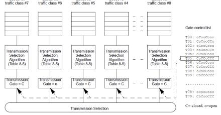
Figure 8-12—Transmission selection with gates
