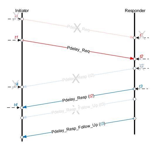
Pdelay measurements as long as Response and Follow Up are received before the next Request is sent. Pdelay measurements occur once per second (AS 11.5.2.2).
