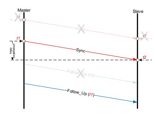
long as it occurs before the next Sync is sent, which is 8 times per second (AS 10.6.2.3, 11.5.2.3). The longer it takes the more "stale" the time is. Therefore, Syncs and Follow\_Ups can communicate time in a collision environment.
