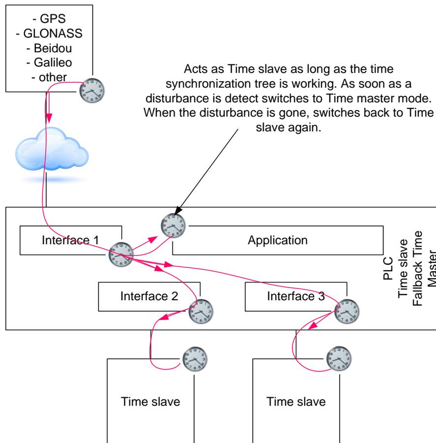
Figure 2 – Synchronization tree for Time
