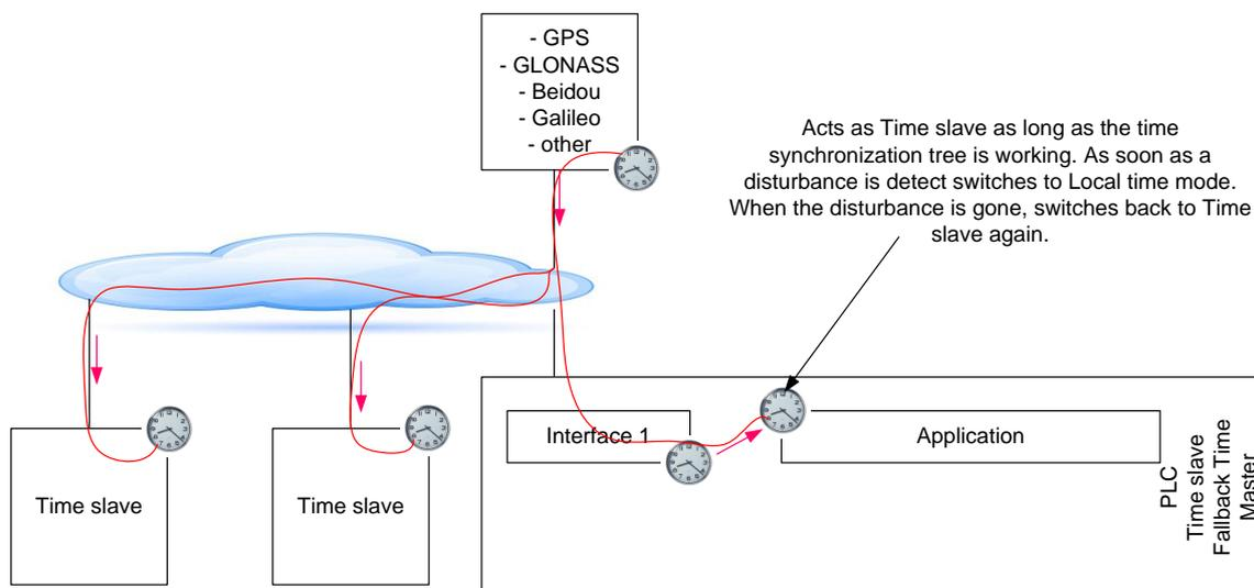
**Figure 6 – Synchronization tree for Time**
