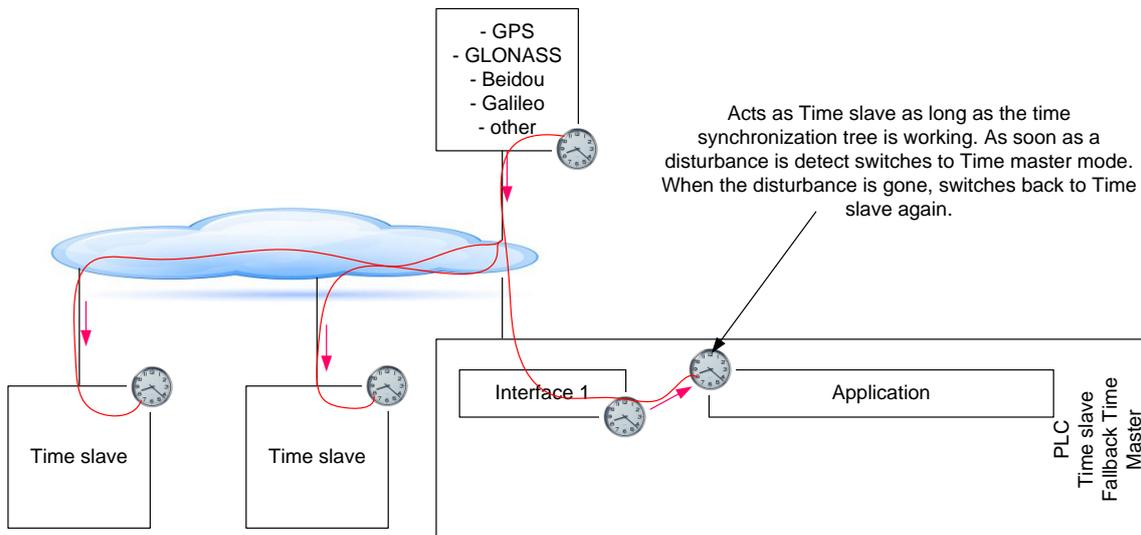
Figure 4 – Synchronization tree for Time
