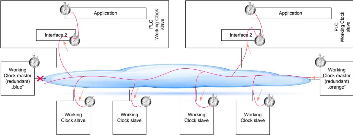
Figure 15 – Broken synchronization tree for "blue" Working Clock
