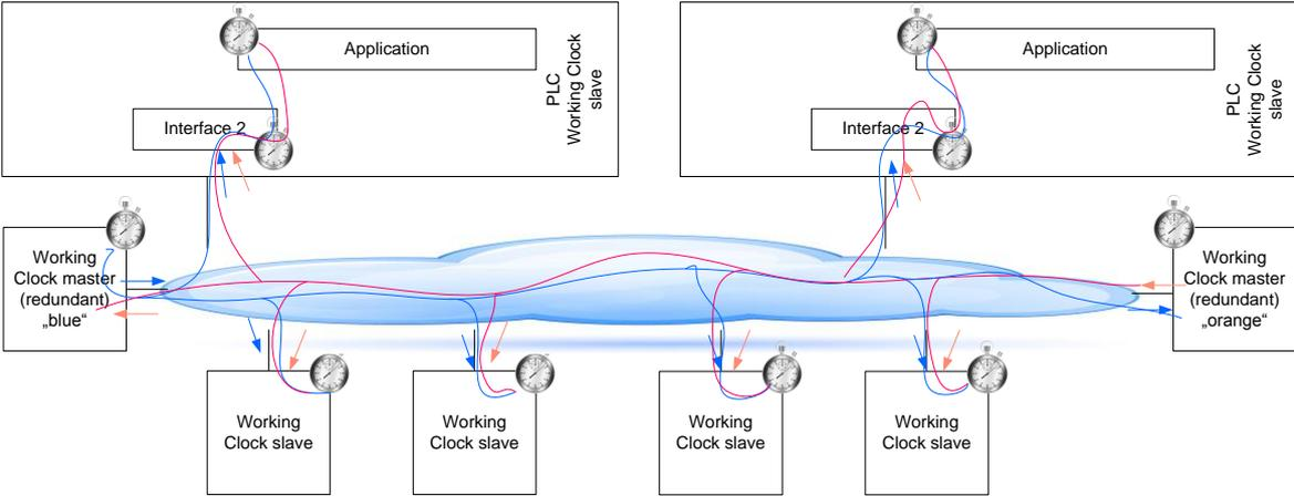
Figure 14 – Synchronization tree for redundant Working Clock
