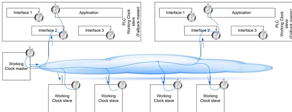
**Figure 10 – Synchronization tree for Working Clock**
