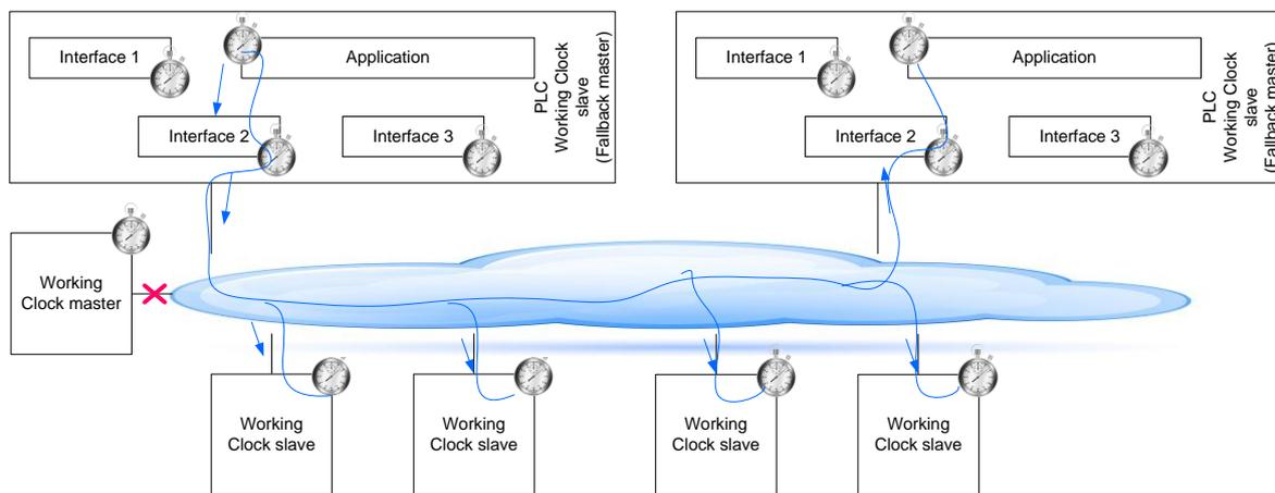
**Figure 11 – Broken synchronization tree with “switchover” SyncMaster for Working Clock**
