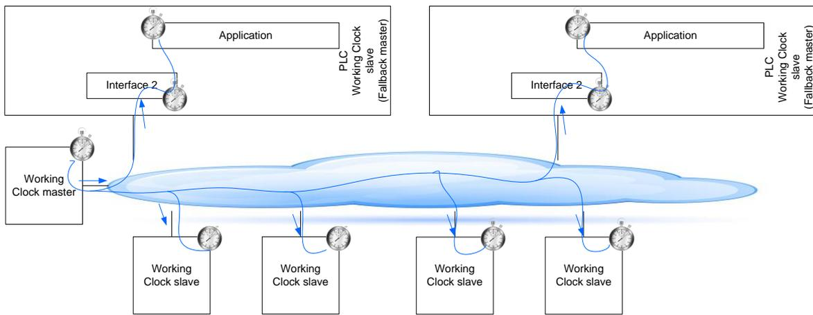
**Figure12 – Synchronization tree for Working Clock**
