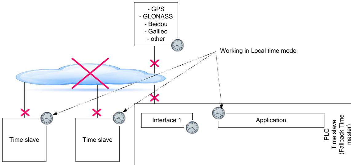
Figure 7 – Broken synchronization tree for Time
