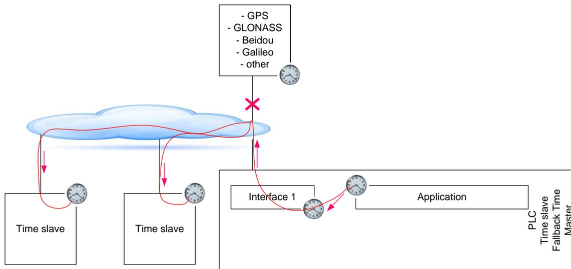
**Figure 5 – Broken synchronization tree for Time**
