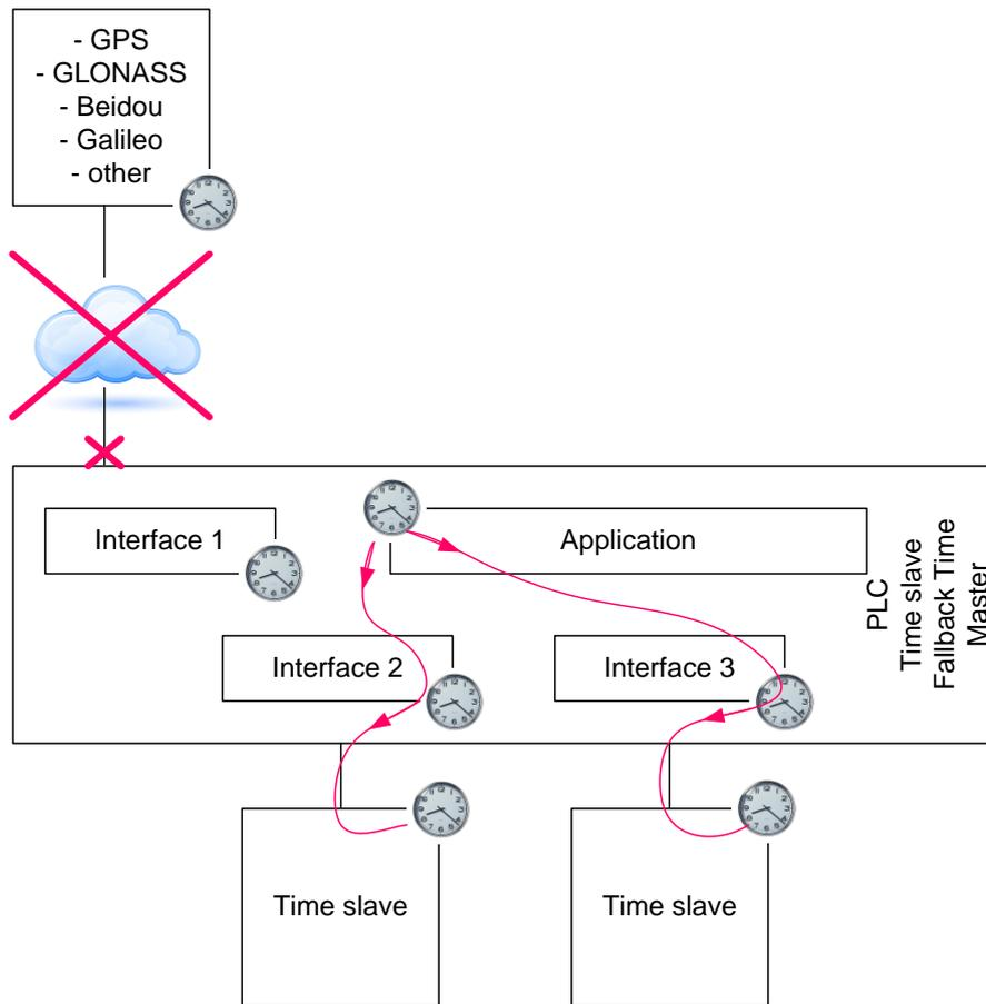
Figure 3 – Broken synchronization tree for Time
