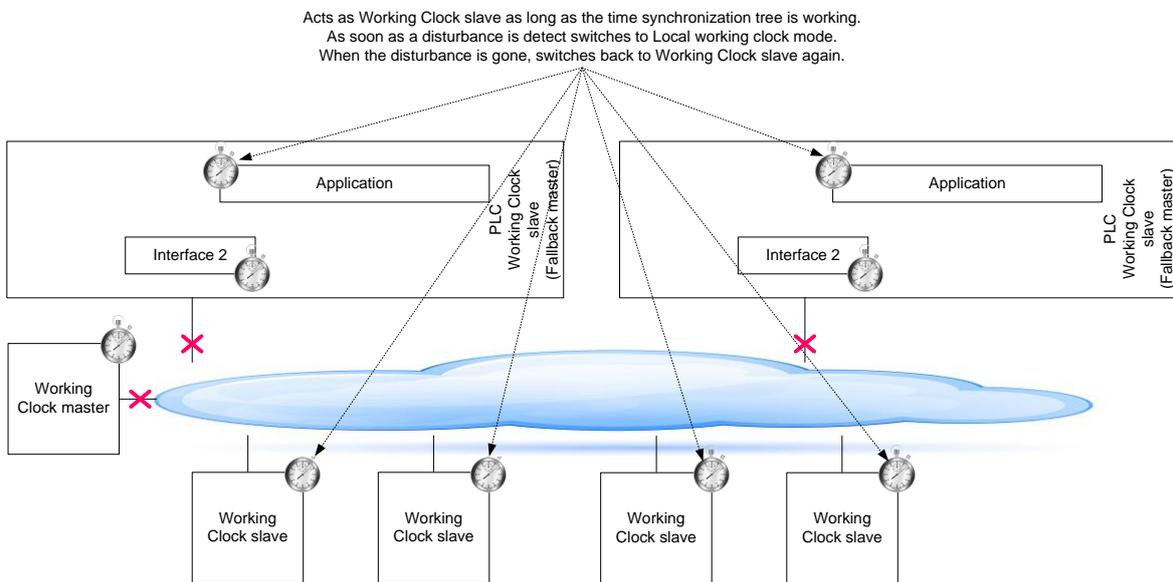
**Figure 13 – Broken synchronization tree for Working Clock**
