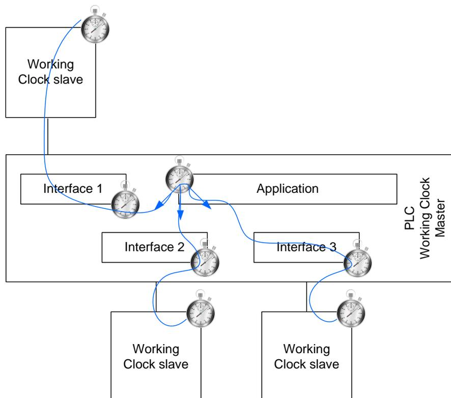
**Figure 9 – Synchronization tree for Working Clock (simple)**
