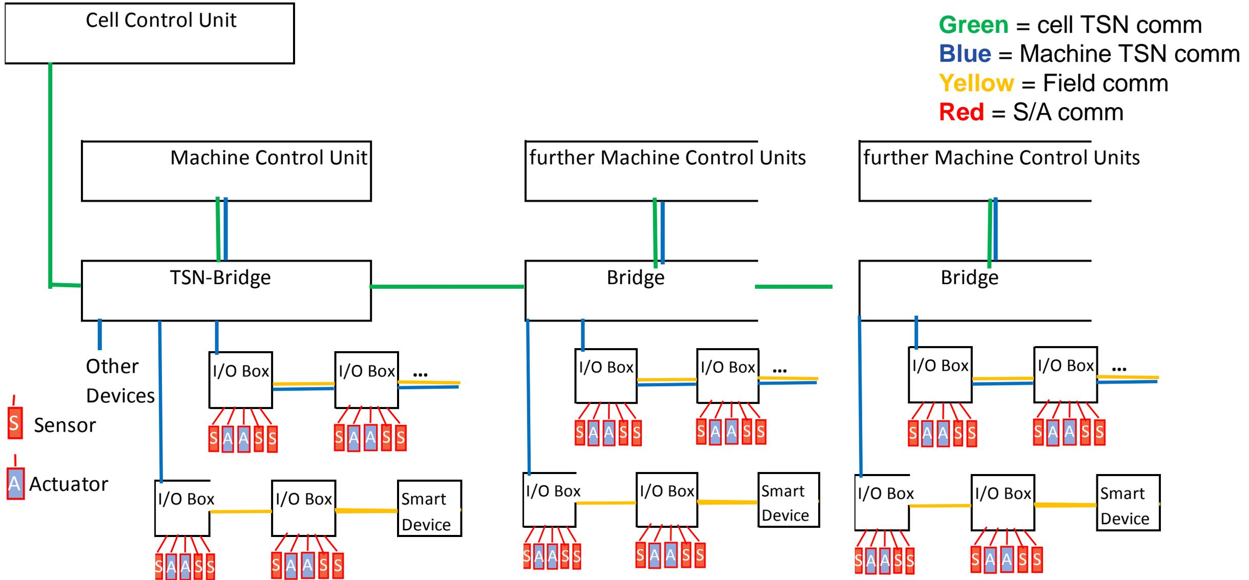
1. The data flow is organized with a **stream** from the **machine control** unit to a (group of) **field devices** and a **stream** from the **field devices** to the **machine control unit**.
