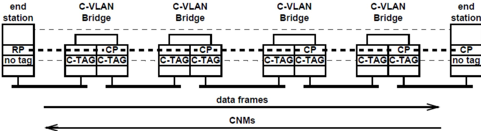
Figure 30-5—CP-RP peering in VLAN Bridged Network
