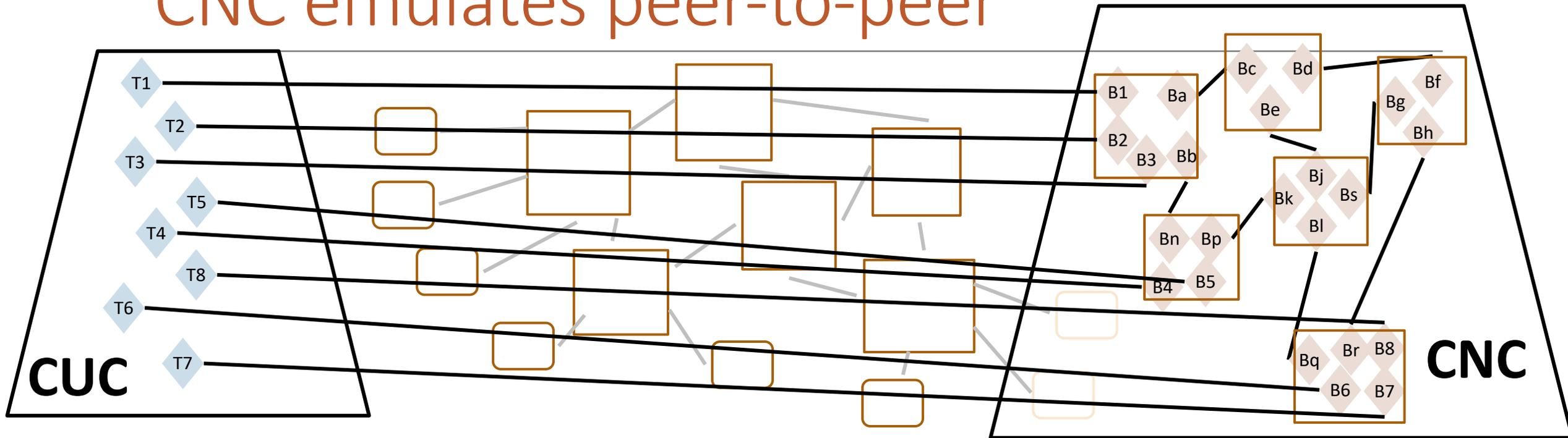
**CUC** controls Talkers, **CNC** controls Bridges.
