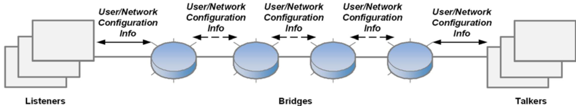
Figure 46-1 — Fully Distributed Model
