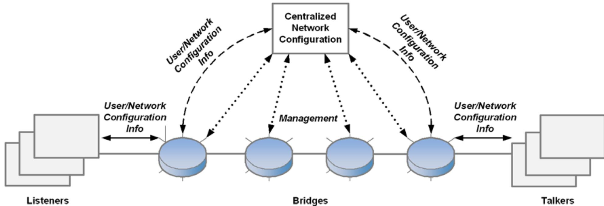
Figure 46-2 — Centralized Network / Distributed User Model
