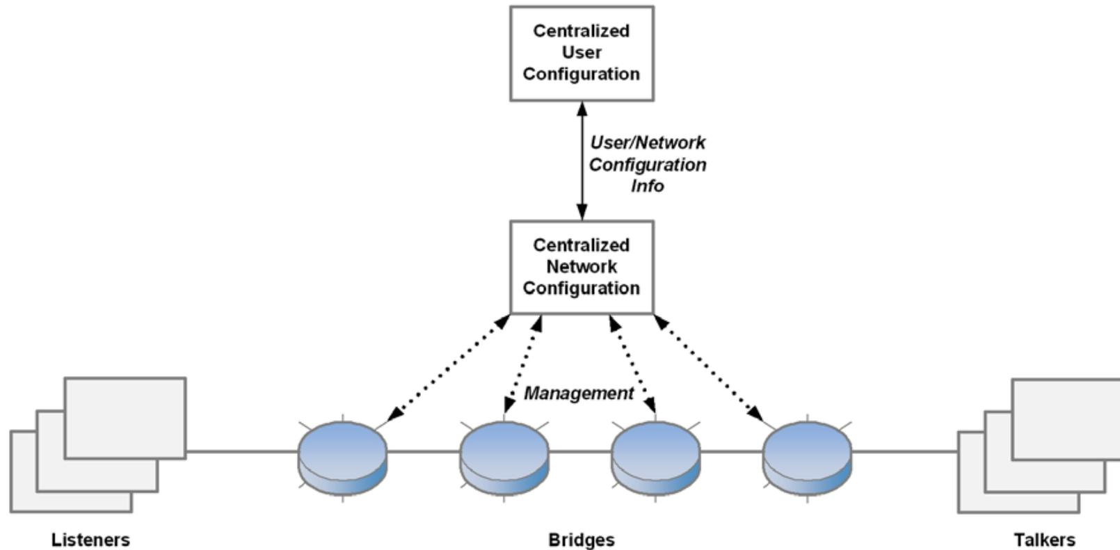
Figure 46-3 — Fully Centralized Model
