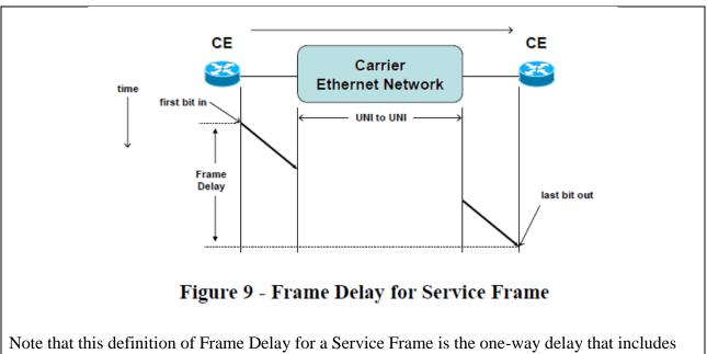
the delays encountered as a result of transmission of the Service Frame across the ingress and egress UNIs as well as that introduced by the CEN.
