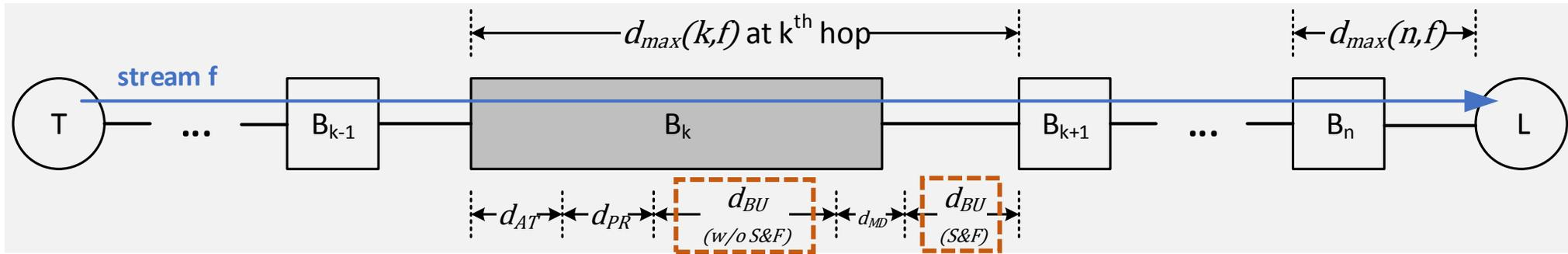
▪ **Delay bound at  $k^{\text{th}}$  hop for stream  $f$ :**  $d_{max}(k, f) = d_{AT,max}(k) + d_{PR,max}(k) + \mathbf{d_{BU,max}(k, f)} + d_{MD,max}(k)$
