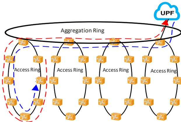
Use \*Network Calculus methodology to setup traffic model and network model and evaluate the latency performance.
