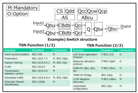
L2 Column shows in diagram of TSN functions.
