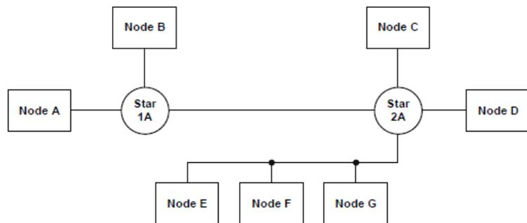
Figure 10 — Single channel hybrid example
