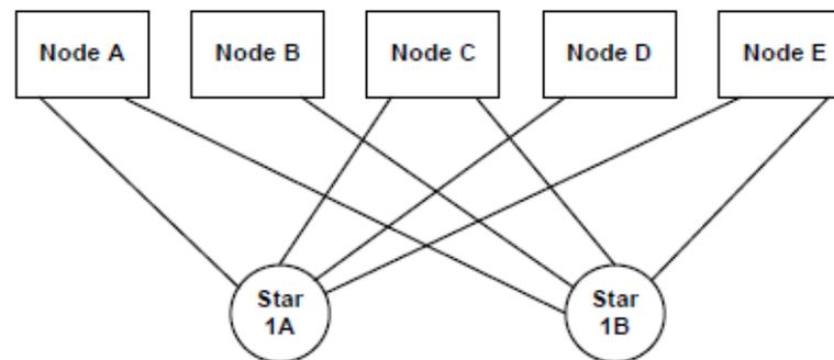
Figure 7 — Dual channel single star configuration
