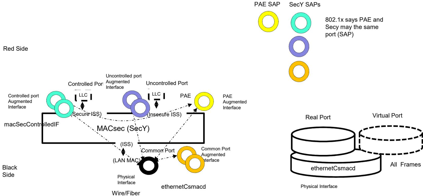
Slightly Different 802.1X Model No Virtual Interface One PAE instance
