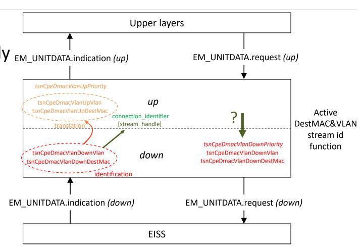
How to determine the set of replacement parameters to use down the stack
