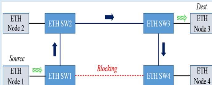
RSTP operation with network failure
