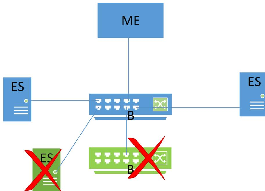
Figure 4: Simple TSN Domain – remove a device
