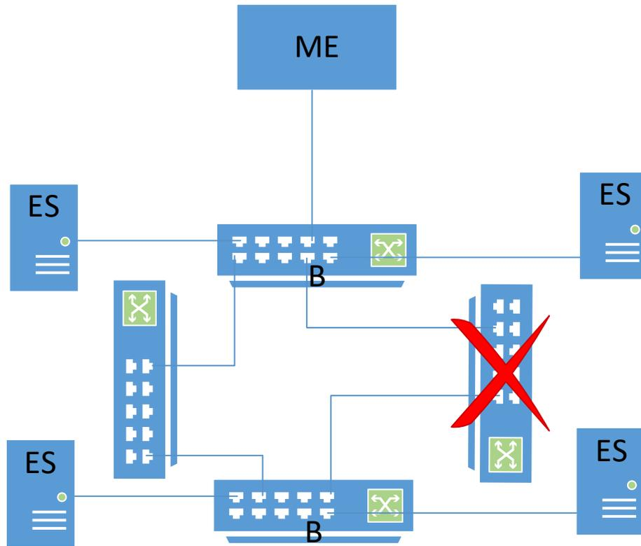
Figure 7: Simple ring topology – one fault
