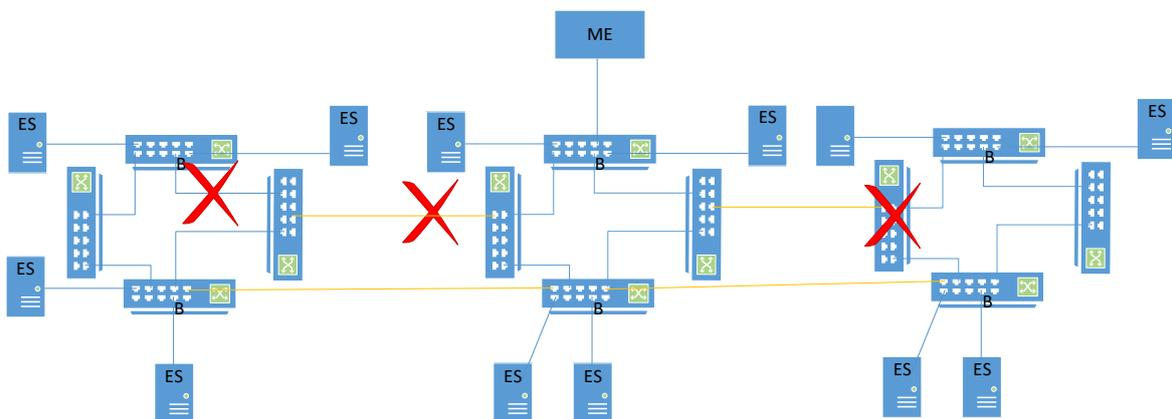
Figure 8: Coupled rings topology – multiple faults
