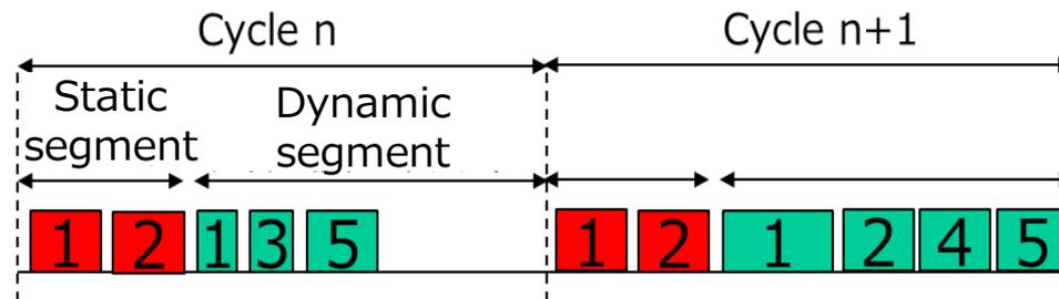
Static segment: Static TDMA is used to arbitrate transmissions.
