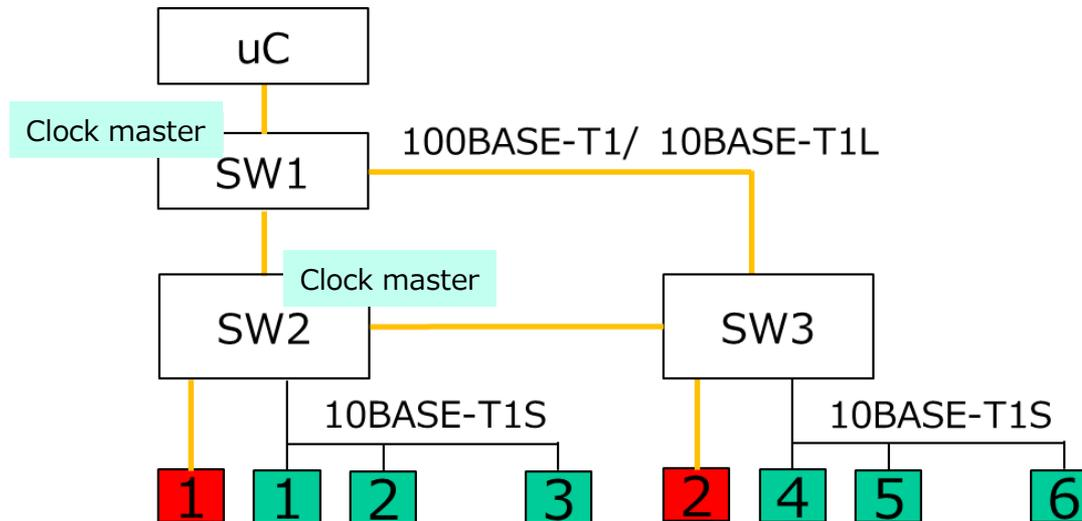
\* The impossibility of Startup at failure of a bridge or a clock master is allowable, the redundancy of clock master and redundant path for time-synchronization are not necessary.
