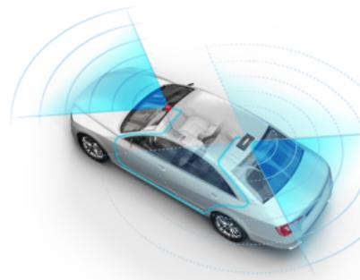
~ 10ms E2E network latency required to avoid collision based on 3 – 27 Mbps application signal rate
