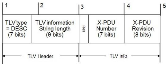
Figure 5: Extension PDU Identifier TLV (XID TLV) Format
