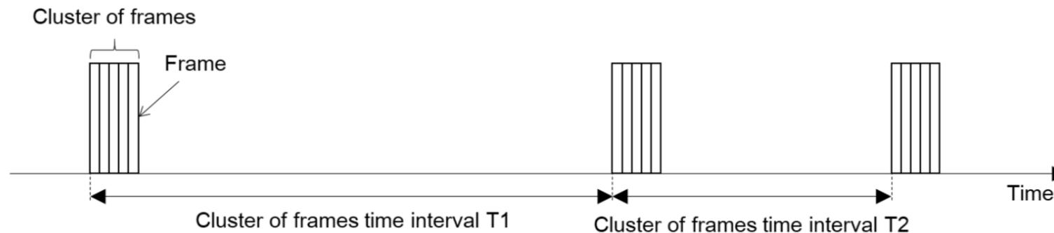
**Figure Z-1— Example of bursty traffic pattern**
