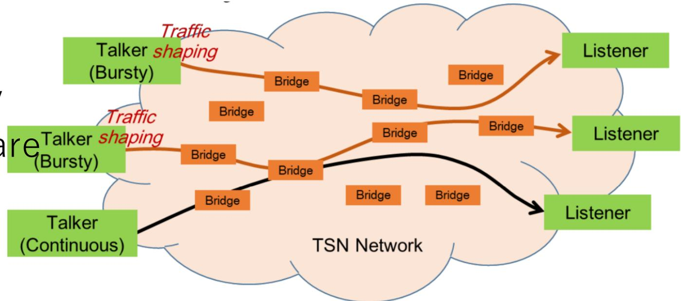
Figure Z-2 — An example of network structure under consideration
