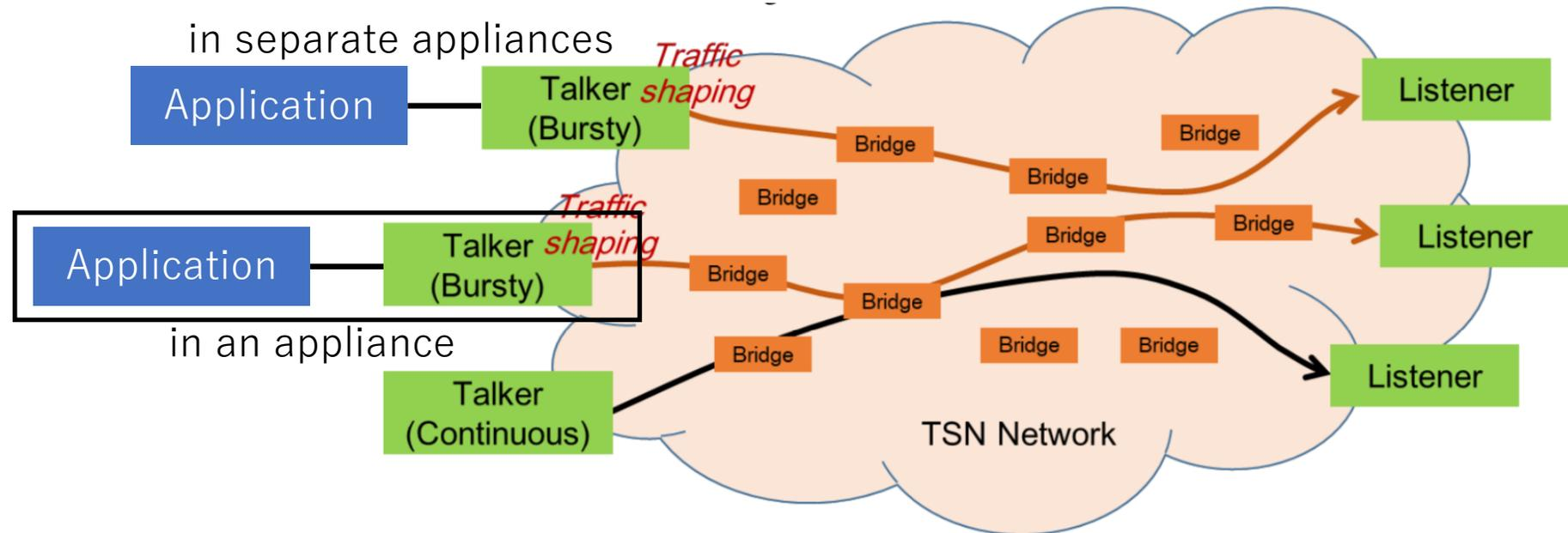
Figure Z-2 — An example of network structure under consideration
