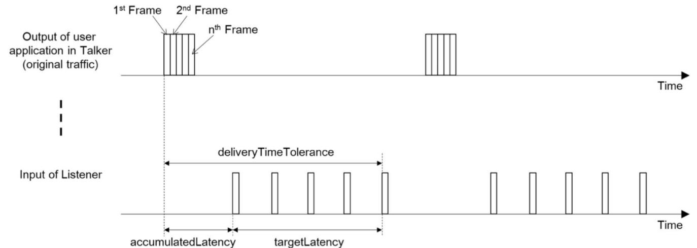
Figure Z-4— Frame propagation within delivery time tolerance while minimizing over-provisioning of bandwidth reservation
