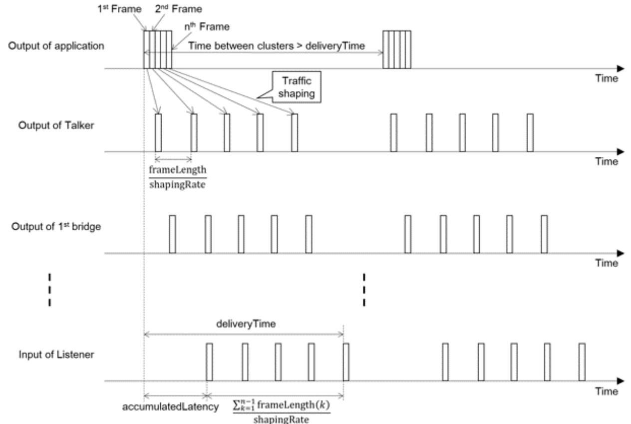
Figure Z-3— Frame propagation from Talker to Listener
