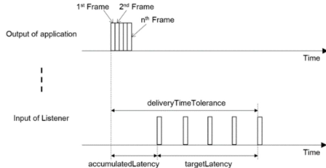
Figure Z-4— Frame propagation within delivery time tolerance while minimizing over-provisioning of bandwidth reservation
