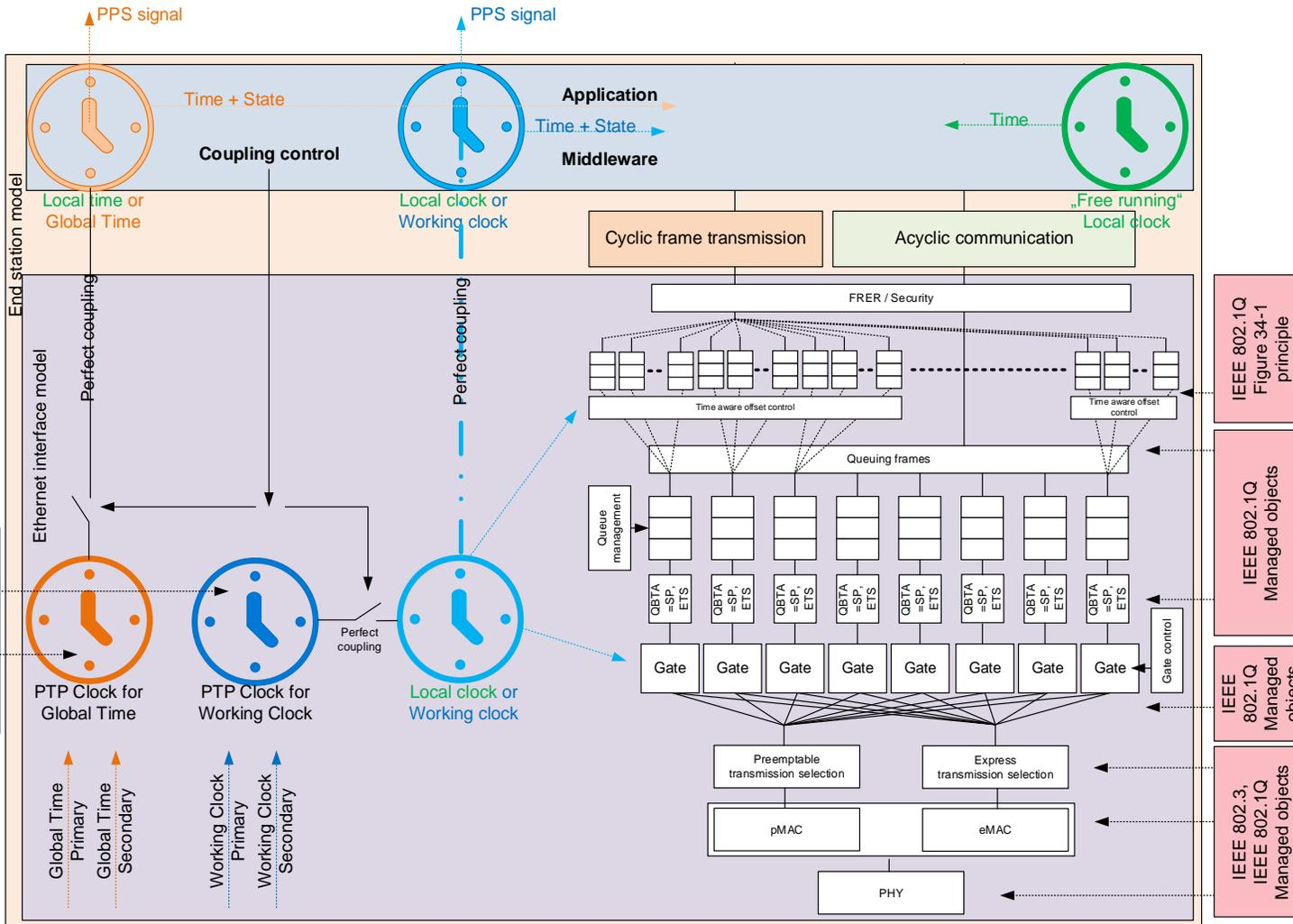
The end station interface and end station model needs to include synchronization.
