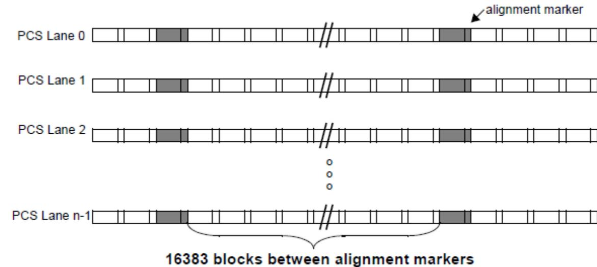
Figure 82-8—Alignment marker insertion period
