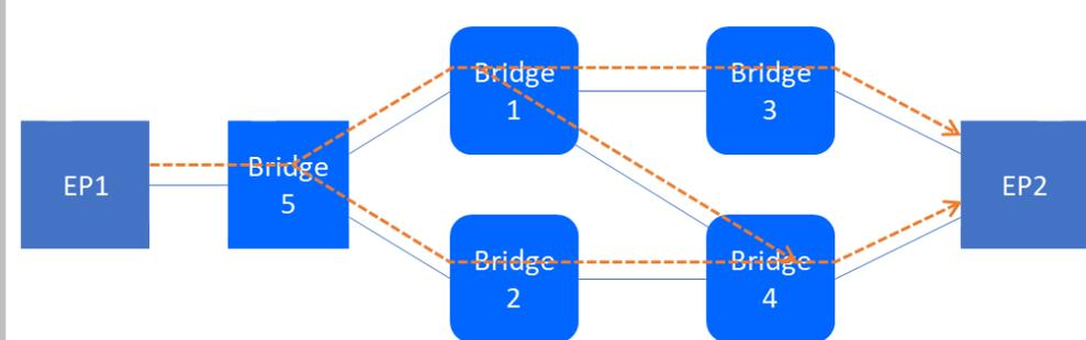
Flexible Positioning of CB functions. EP1 is not CB capable, EP2 is CB Capable
