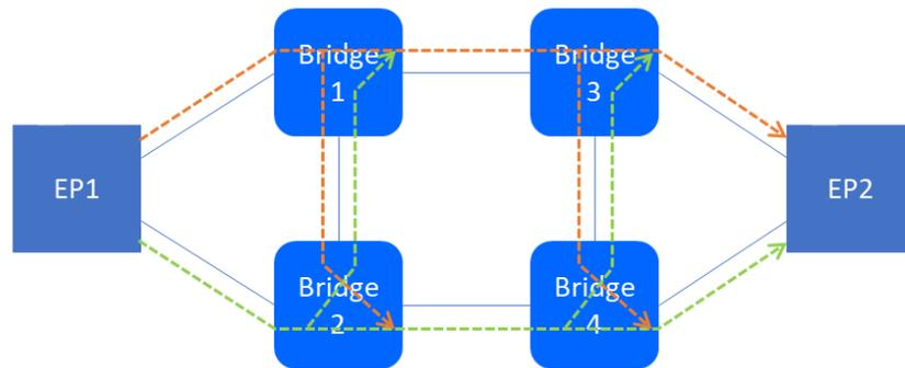
Ladder Redundancy: Resistant to multiple link failures
