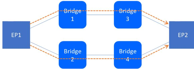
CB Capable, Dual Homed End Points using Link Aggregation
