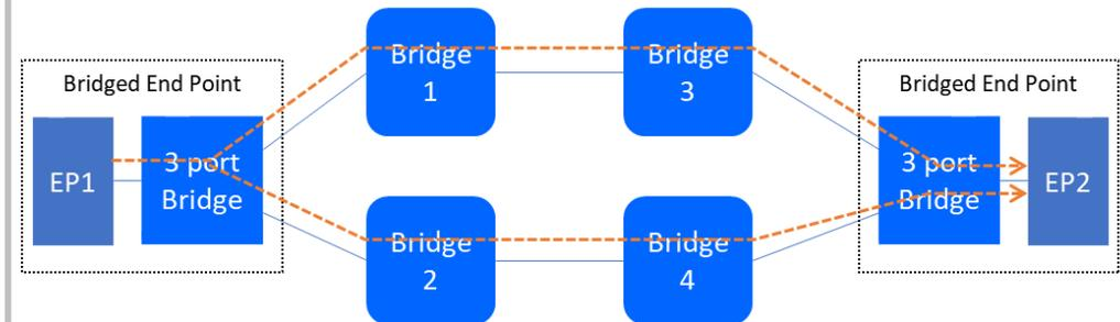
Bridged End Points. EP1 is no CB capable, EP2 is CB Capable
