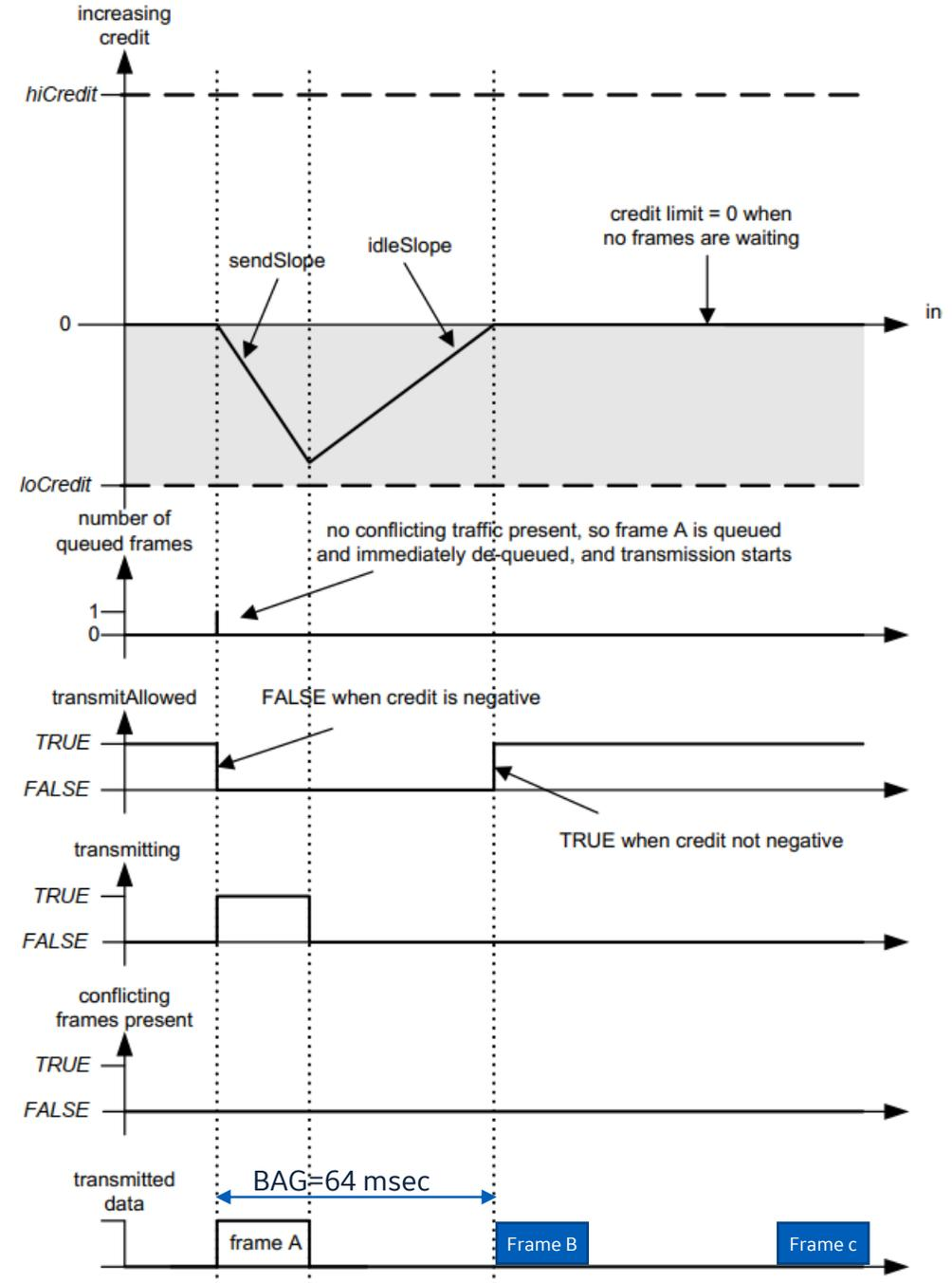
Figure L-1—Credit-based shaper operation—no conflicting traffic
