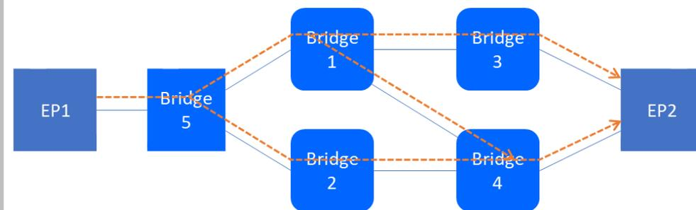
Flexible Positioning of CB functions. EP1 is not CB capable, EP2 is CB Capable
