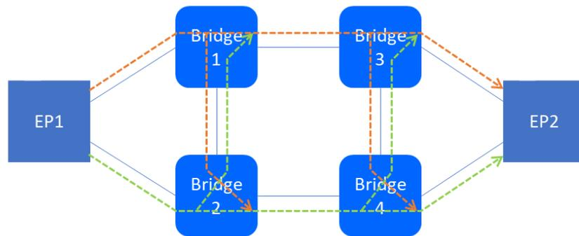
Ladder Redundancy: Resistant to multiple link failures
