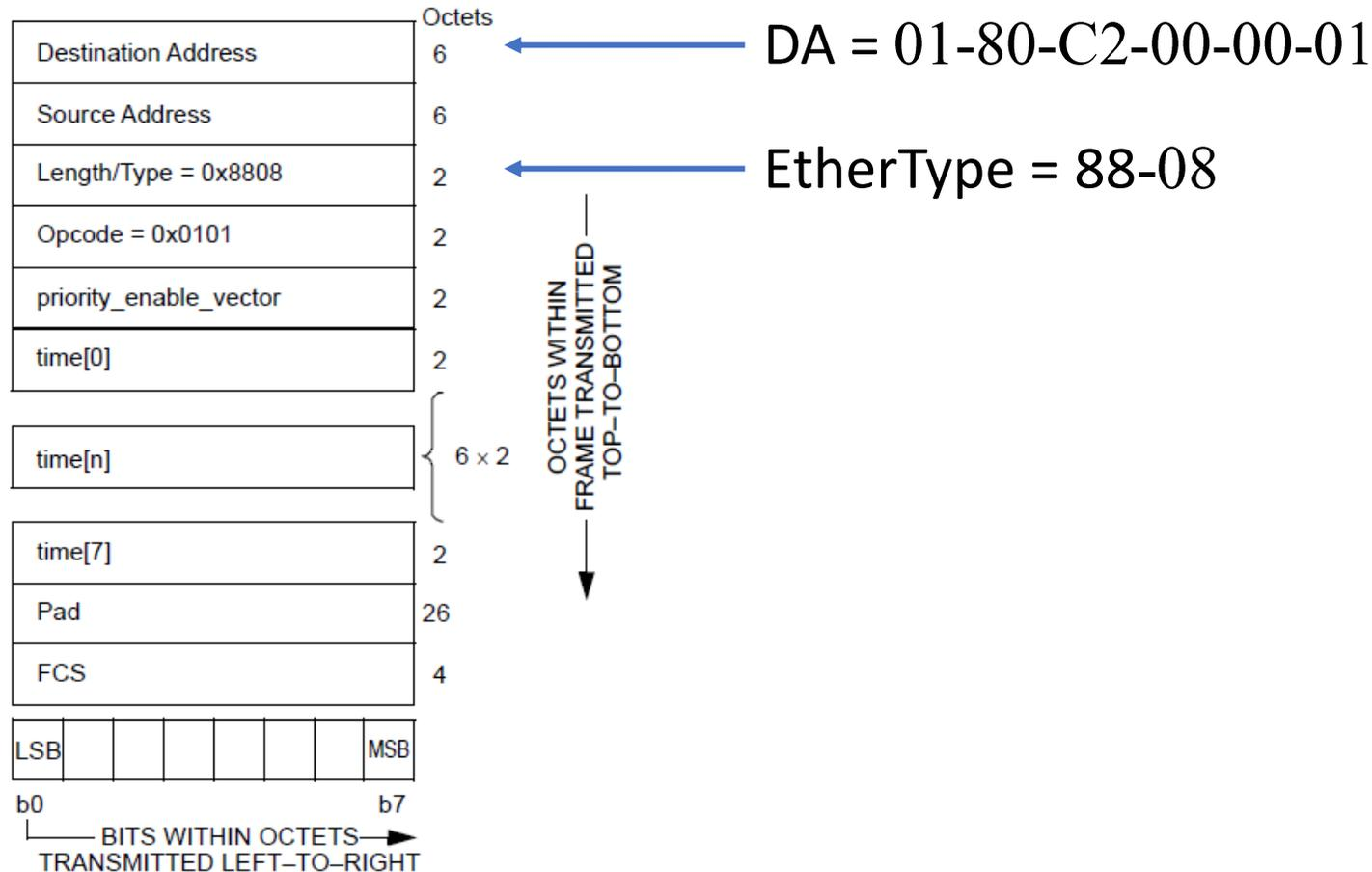
Figure 31D-1—MAC Control EXTENSION Frame
