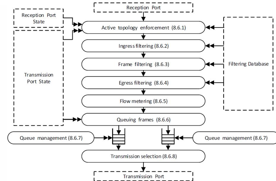
Figure 8-12—Forwarding process functions
