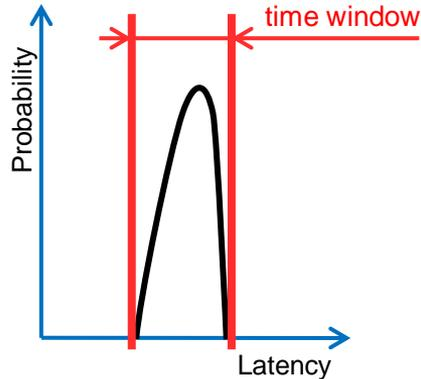
TSN is a set of standards specified by IEEE 802 to provide deterministic data transfer in packet networks, e.g., in Layer 2 bridged networks
