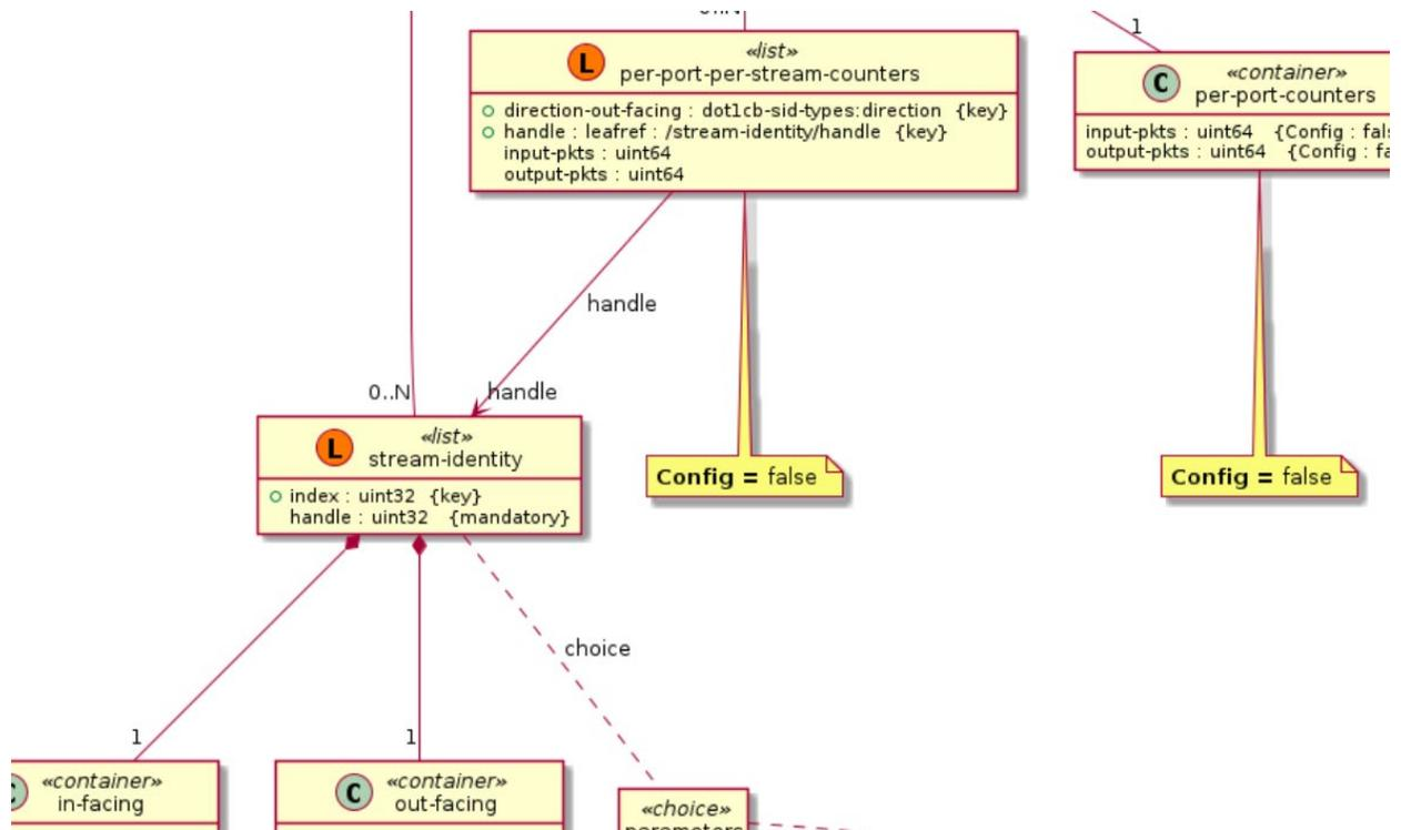
Figure 5 - Detail of ieee802-dot1cb-stream-identification.yang
