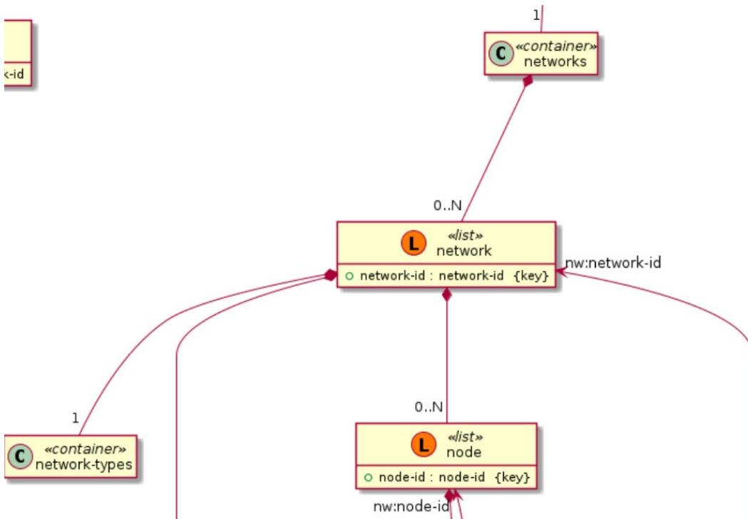
Figure 3 - Detail of ietf-network.yang uml-like diagram
