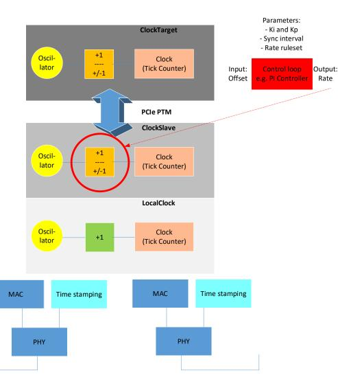
Each calculated Offset value (time interval e.g. in nanoseconds) is used as an input for a PI controller which calculates the "new" rate controlling the ClockSlave time.
