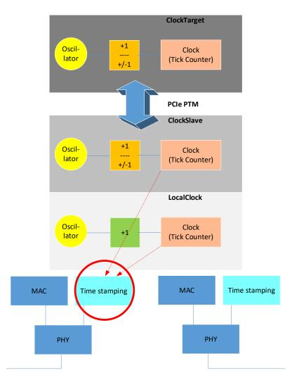
The rate ratio between the ClockMaster and the ClockSlave can be calculated in multiple ways.
