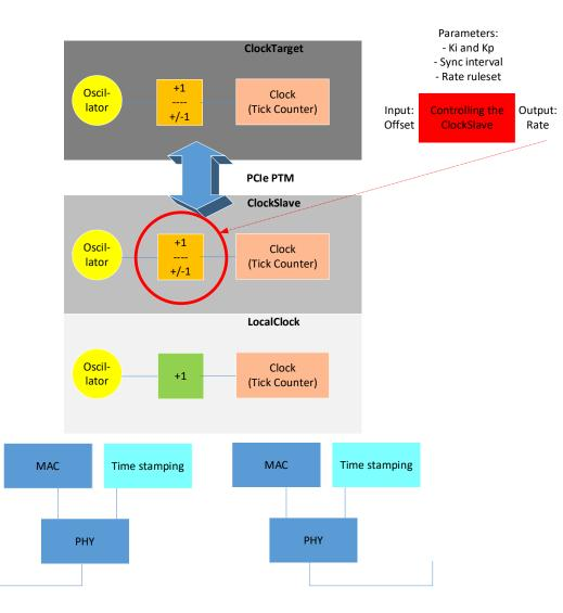
Each calculated Offset value (time interval e.g. in nanoseconds) is used as an input for a PI controller which calculates the "new" rate controlling the ClockSlave time.
