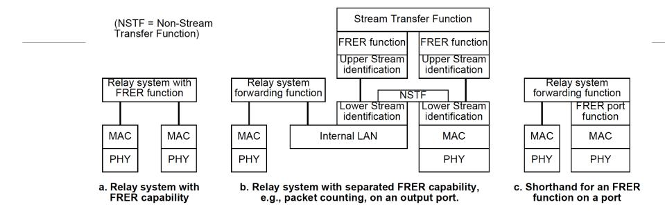
Figure 6-5—Stream functions in a relay system (three views of same system)
