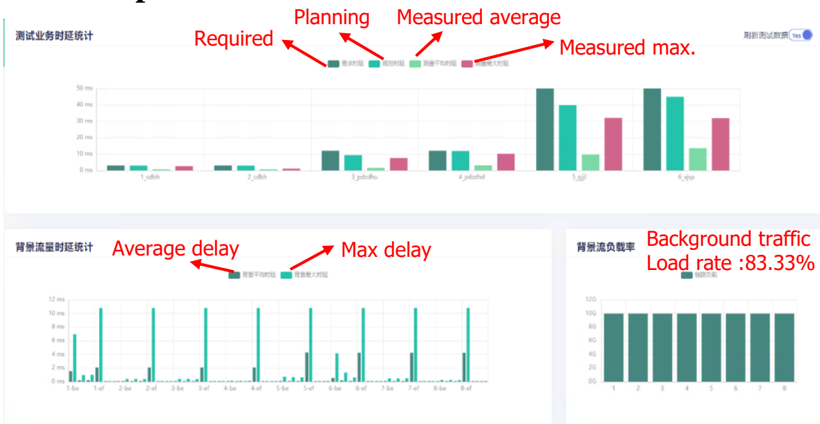
Figure: TSN-IP SLA guarantee effect in smart grid scenario
