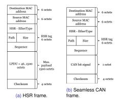
Figure 2: Comparison between a standard HSR and Seamless CAN frame.
