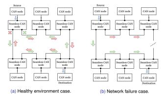
Figure 4: Single-ring Seamless CAN network in two environments.
