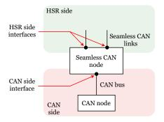
Figure 3: Seamless CAN node's interfaces.
