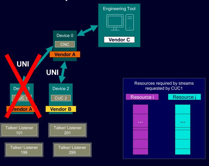
Example 1: CNC-unaware removal of machine controlled by CUC 1
