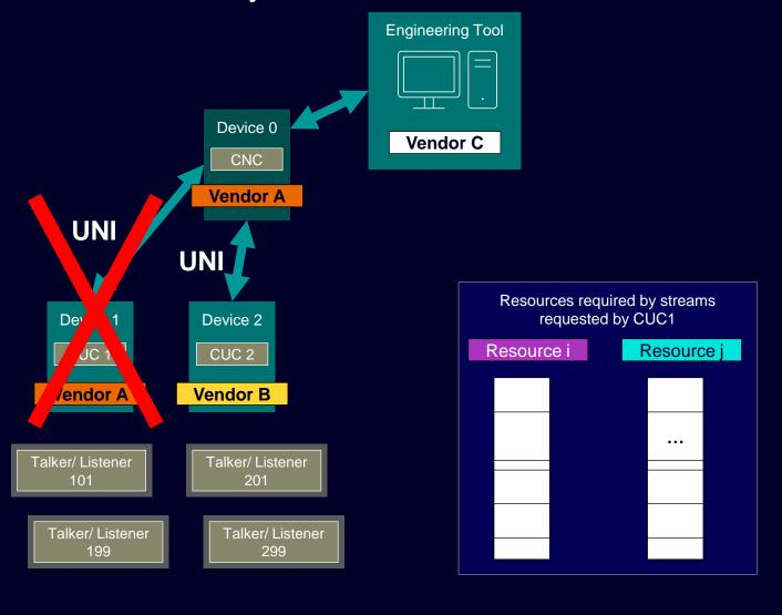
Example 2 : CNC-aware removal of machine controlled by CUC 1
