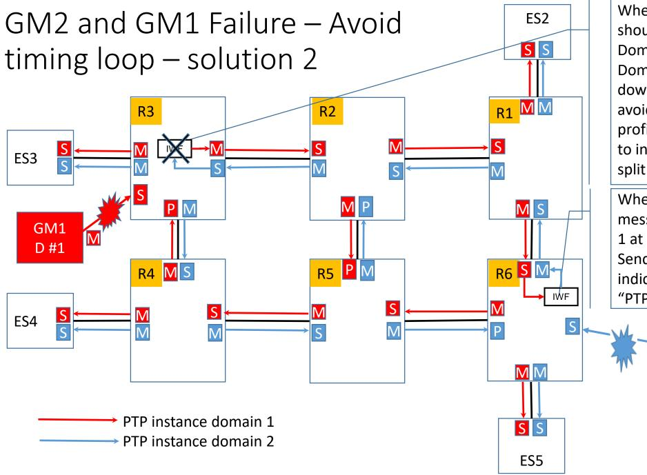
When GM1 fails, R3 knows that it should not activate the IWF as Domain 2 was using time from Domain 1, **send some** information downstream that can be used to avoid the timing loop (e.g. PTP profileSpecific 1" flag can be defined to inform PTP instances that the split function was used upstream.
