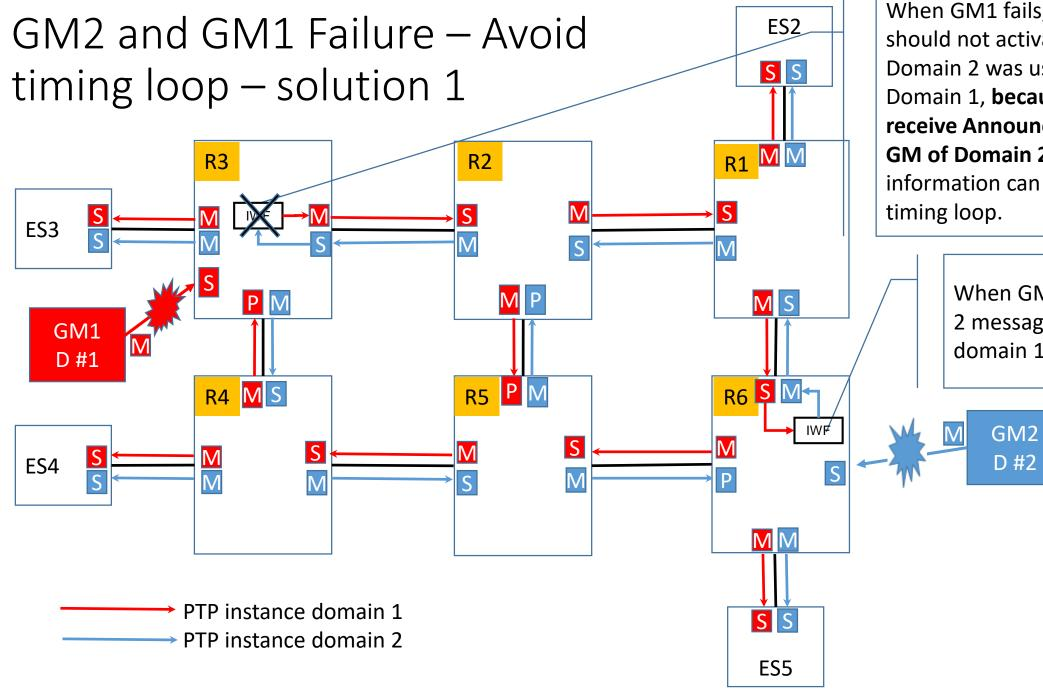
When GM1 fails, R3 knows that it should not activate the IWF as Domain 2 was using the time from Domain 1, **because it does not receive Announce message from the GM of Domain 2**, and therefore this information can be used to avoid the timing loop.
