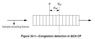
Let Q denote the instantaneous queue size and  $Q_{old}$  denote the queue size when the last feedback message was generated. Let  $Q_{off} = Q - Q_{eq}$  and  $Q_{\delta} = Q - Q_{old}$ .
