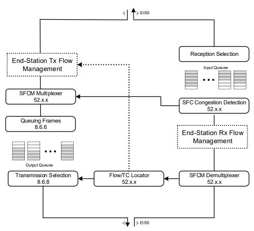
Figure 52-3—End station SFC reference diagram
