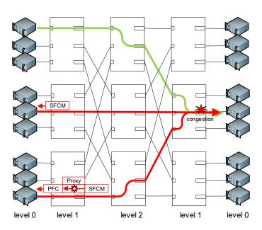
Figure 52-1—Source flow control example operation
