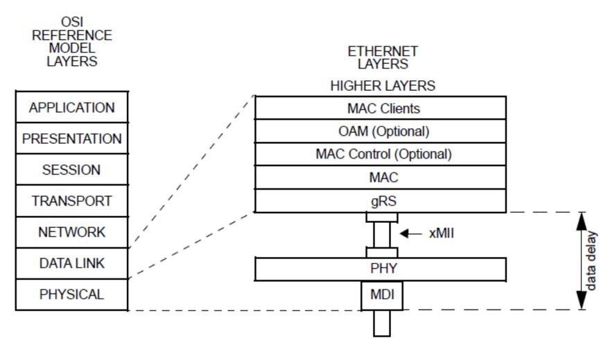
Figure 90-5—Data delay measurement
