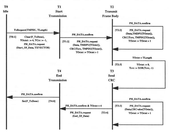
Figure 6-xx(8): Transmitter State Machine
