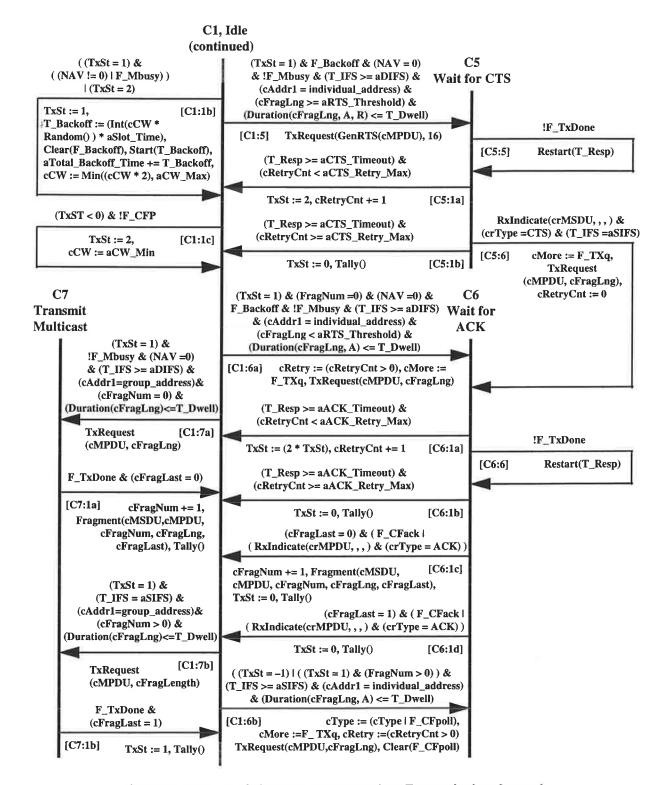
Figure 6-xx(7): MAC Control State Machine, Transmission Control
