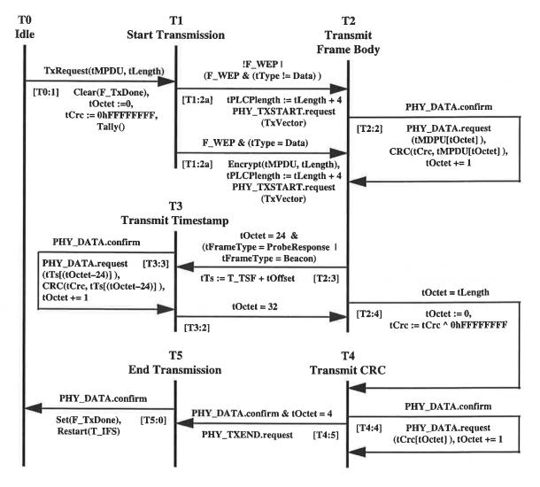
Figure 6-xx(11): Transmitter State Machine
