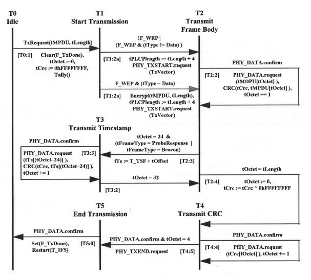
Figure 6-xx(11): Transmitter State Machine
