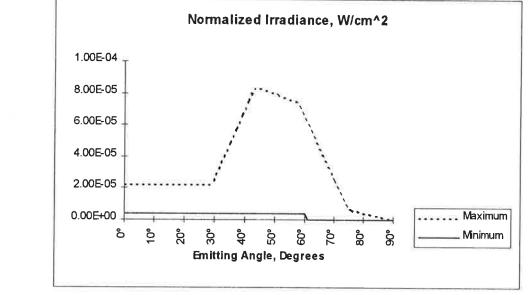
Figure 12-4: Emitter radiation pattern mask.
