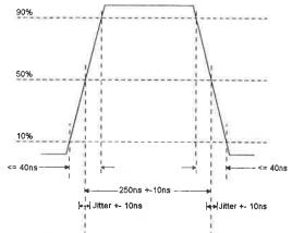
Figure 12-3: Basic Pulse Shape
