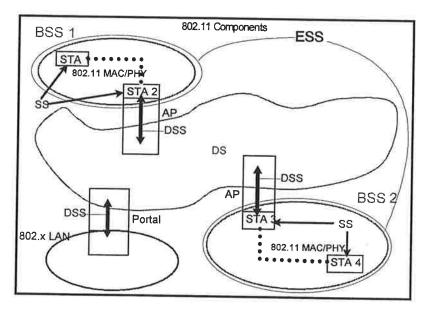
Figure 2-7: Complete 802.11 Architecture
