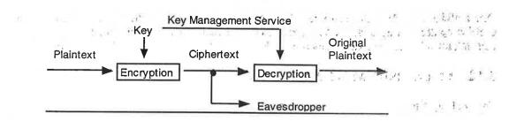
Figure 5-21: A Confidential Data Channel
