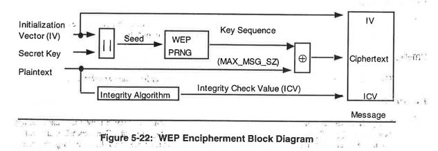
Referring to Figure 5-22 and following from left to right, encipherment begins with a secret key that has been distributed to cooperating stations by an external key management service. WEP is a symmetric algorithm in which the same key is used for encipherment and decipherment.
