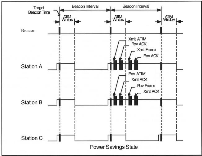
Figure 7-6: Ad Hoc Power Management - Basic Operation
