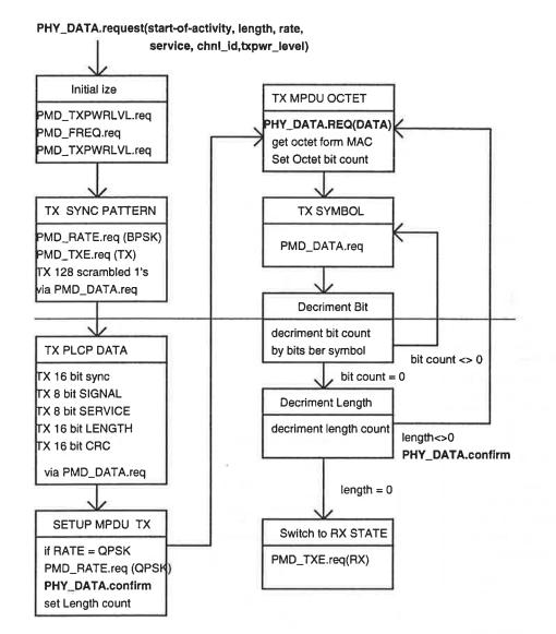
Figure 12-6: PLCP Transmit State Machine
