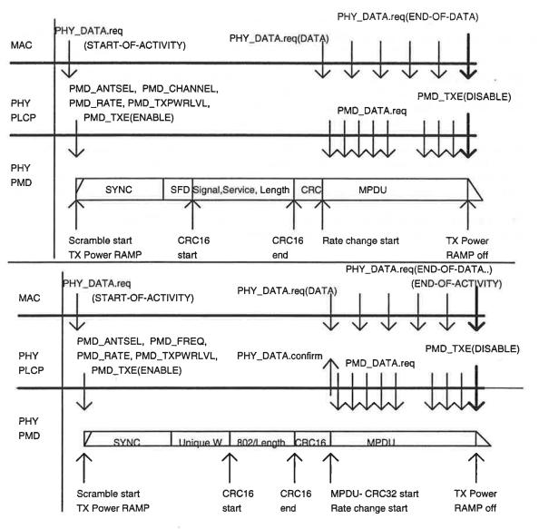
Figure 12-5: PLCP Transmit Procedure
