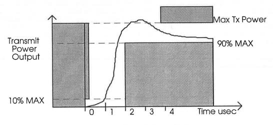
Figure 12-11: Transmit Power On Ramp
