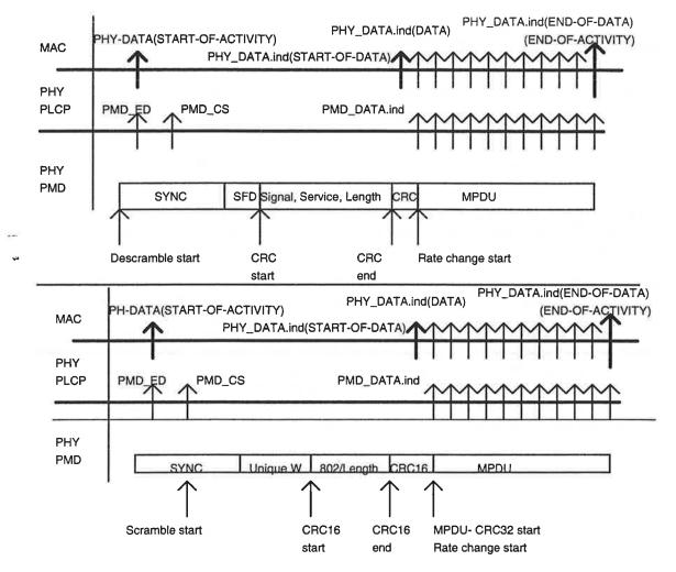
Figure 12-7: PLCP Receive Procedure
