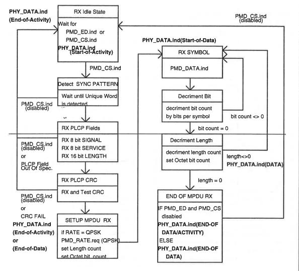
Figure 12-8: PLCP Receive State Machine
