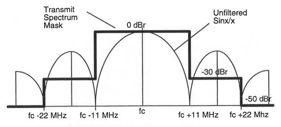
Figure 12-10: Transmit Spectrum Mask
