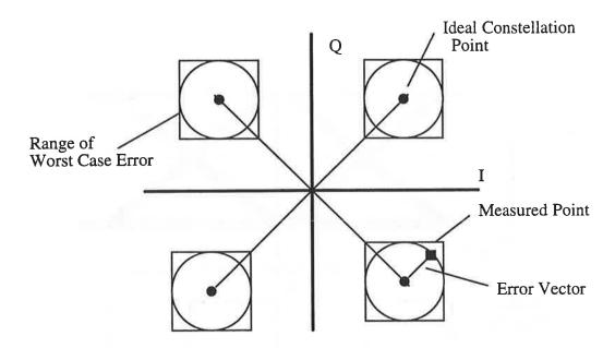
Figure 12-13: Modulation Accuracy Measurement Example
