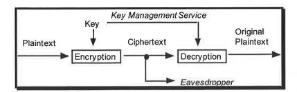
Figure 5-1: A Confidential Data Channel
