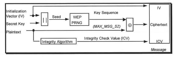
Figure 5-2: WEP Encipherment Block Diagram
